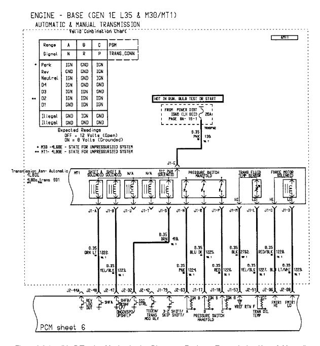
Figure 3.2.1a - IV - P/Truck - Mechanization Diagram - Engine to Transmission (Auto & Manual)
